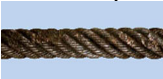
Heat, Chemical or Electrical damage
